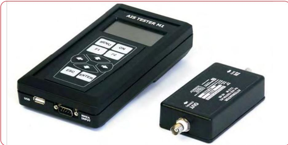
Thus the AIS tester can be easily connected to any PC or laptop. The connection is carried out by means of standard USB A-USB A cable and special software available on this website. The minimal requirements are Microsoft OS, such as Windows XP, Windows Vista or Windows 7 and USB port. No special hardware configuration is required.
