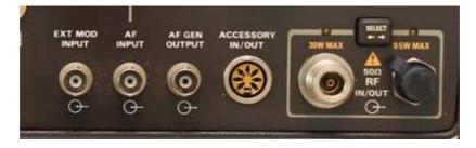
Example EXT modulation input on "Marconi 2955: Radio communications Test Set"
