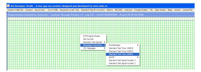
Set the modulation frequency to 1KHz and zero level / deviation.
