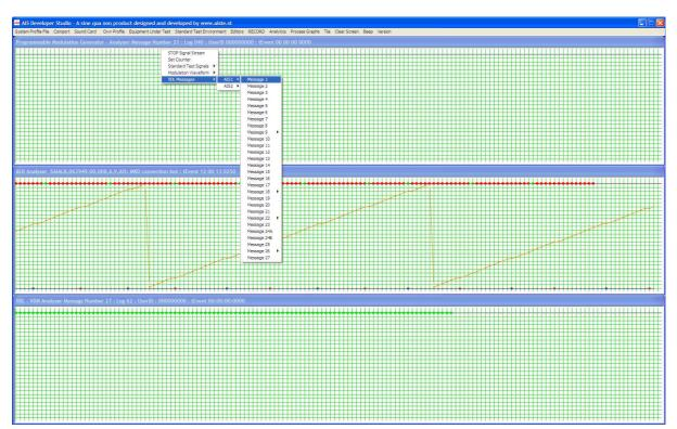
The selection of AIS1 or AIS2 will change the channel indication of the Programmable Modulation Generator VDO string.
