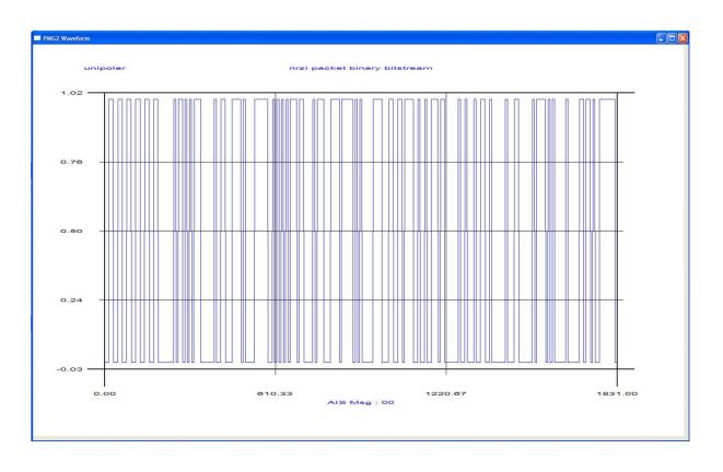
NRZI initial state for packet 3, and packet 4 in sequence = 1
